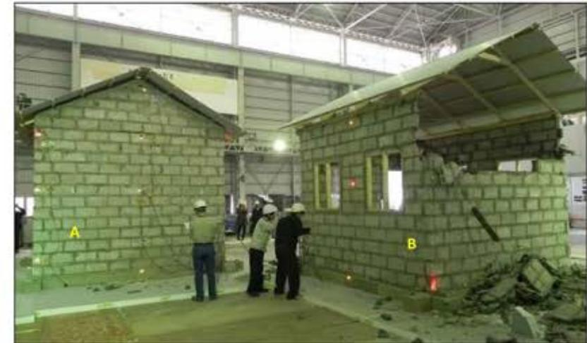
*Picture shows the collapsed gable part of the back wall of model B*
