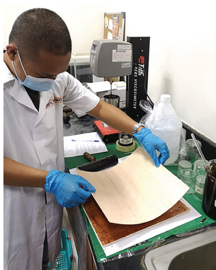
Plywood production using tannin-phenol formaldehyde adhesive.
