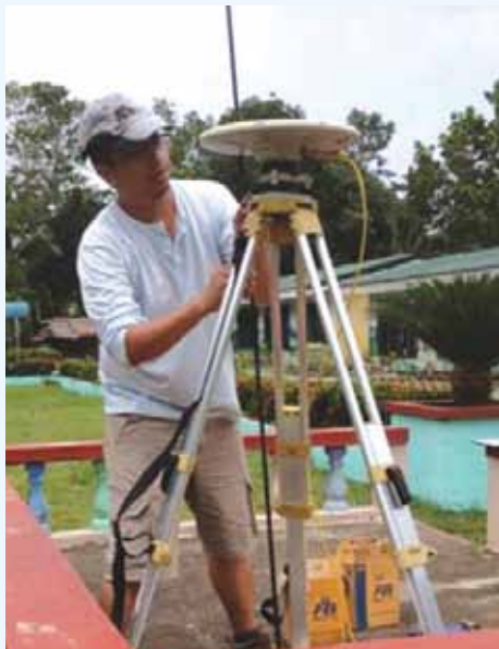
Teresito Bacolcol during a GPS survey in Matalam, Cotabato to assess the post-seismic deformation associated with the June 2013 Ms 5.7 earthquake in Cotabato.
