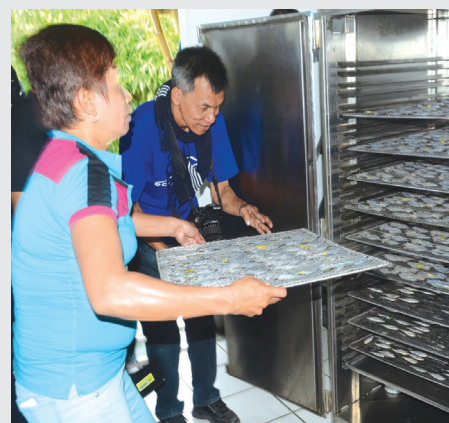
Solar-powered fish dryer (Photos by Gerardo G. Palad, S&T Media Service, DOST-STII)
