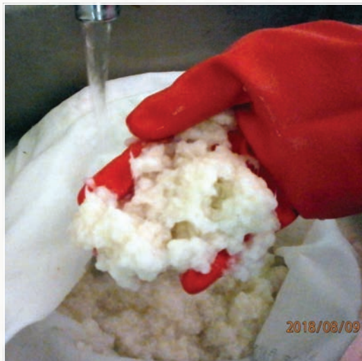
Bleached abaca pulp will be converted into cellulose nitrate, a main ingredient of propellants.
