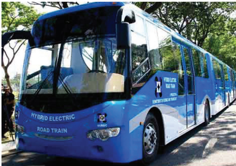
The Hybrid Electric Road Train is an alternative mass transport system that was developed by the DOST-Metals Industry Research and Development Center.
