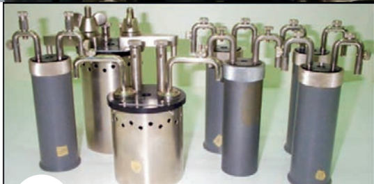
Calibration of standard resistors at the NML's Electrical Standards Laboratory
