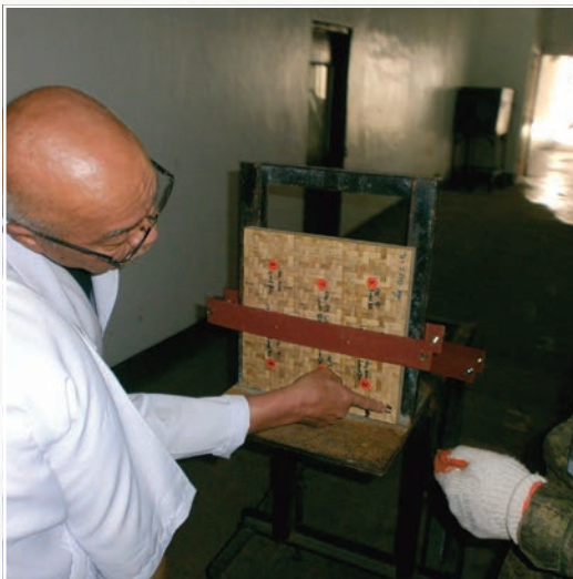
The experimental bamboo mat is tested as possible material for body armors at the Philippine Army R&D Center.
